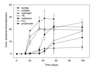
Figure 3. Benzene and chlorobenzene production during dechlorination of β-HCH in soil sample ANC2, stimulated by different electron donors. YE – yeast extract, FLL – fermented landfill leachate.
