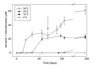
Figure 1. Influence of temperature on the dechlorination of  $\beta$ -HCH. The arrow on day 62 indicates when the culture incubated at 30 °C was refed with  $\beta$ -HCH and further incubated at 10 °C.
