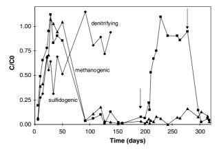
Figure 4. Dechlorination of β-HCH in soil columns under different redox conditions. The HCH concentration is plotted as the concentration in the effluent over the concentration in the influent. The arrow on day 193 marks the replacement of 10 mM sulphate with 10 mM nitrate in the influent; the arrow on day 278 marks the restoration of the original setup.
