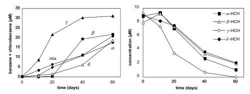
Figure 2. Reductive dechlorination of different HCH isomers in the soil slurry when applied both separately, and as a mixture (top panel, measured as benzene and CB production), and disappearance of the separate HCH-isomers in the mixture (bottom panel).
